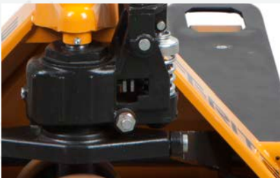
Greaseable bushings ensure a long service life
